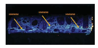
Transpo T-70 has been shown to have penetrating capabilities of over one inch.
